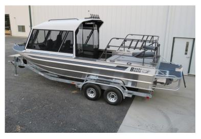
Tietsort 24' propulsion package combines Indmar's Ford Raptor 575 supercharged motor to Hamilton's 241 water jet. Custom upholstery, wrap and flooring throughout makes for a clean, sharp look. Full overhead viewing windows with a center gullwing in the hardtop gives great visibility forward. Custom stereo system, washdown, rear rail corner seats, anchor locker and ski pole are just a few of its amenities.
